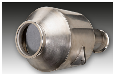
A typical aircraft ozone converter Photo: basf.com
